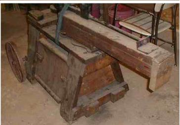
Note the flanking blocks on the rear/lower 2x4. The post rotates down and between those blocks and is held in place with a heavy adjustable 'U' bolt that inserts into holes just forward of the rearmost 2x4. The post is a stack of 4 2x6's onto which a post-vise is bolted The vise mount was modified to fit the post...
