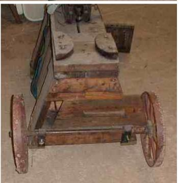
The bench served me well for many years and has only been recently replaced by a trailer assembly. It has the advantage that you can load it with all the tools and bits and pieces you need. You then only need to remember to bring one big item rather than tens of little items. The downside is pushing all the weight up and down a ramp - just make sure the wheels are wide enough to roll over soft ground.
