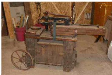
The basic construction is a set of 2x6 legs, flanked by a set of 2x4's (on either side of the leg and at the top and bottom of the leg set) (see pic to right). All are fastened with lag screws and glue. A pair of 2x6's form the top deck and a sheet of plywood runs from the lower surface of the upper 2x4's and from the upper surface of the lower 2x4's to tie the bench together. Sheet material closes off the sides between the legs (the left side cover can be removed for access to the interior)
